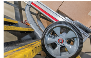
Stair climbers assist with transporting loads up and down stairs
